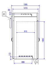
Drain Electrical inlet (power) RO Refrigerant Outlet
